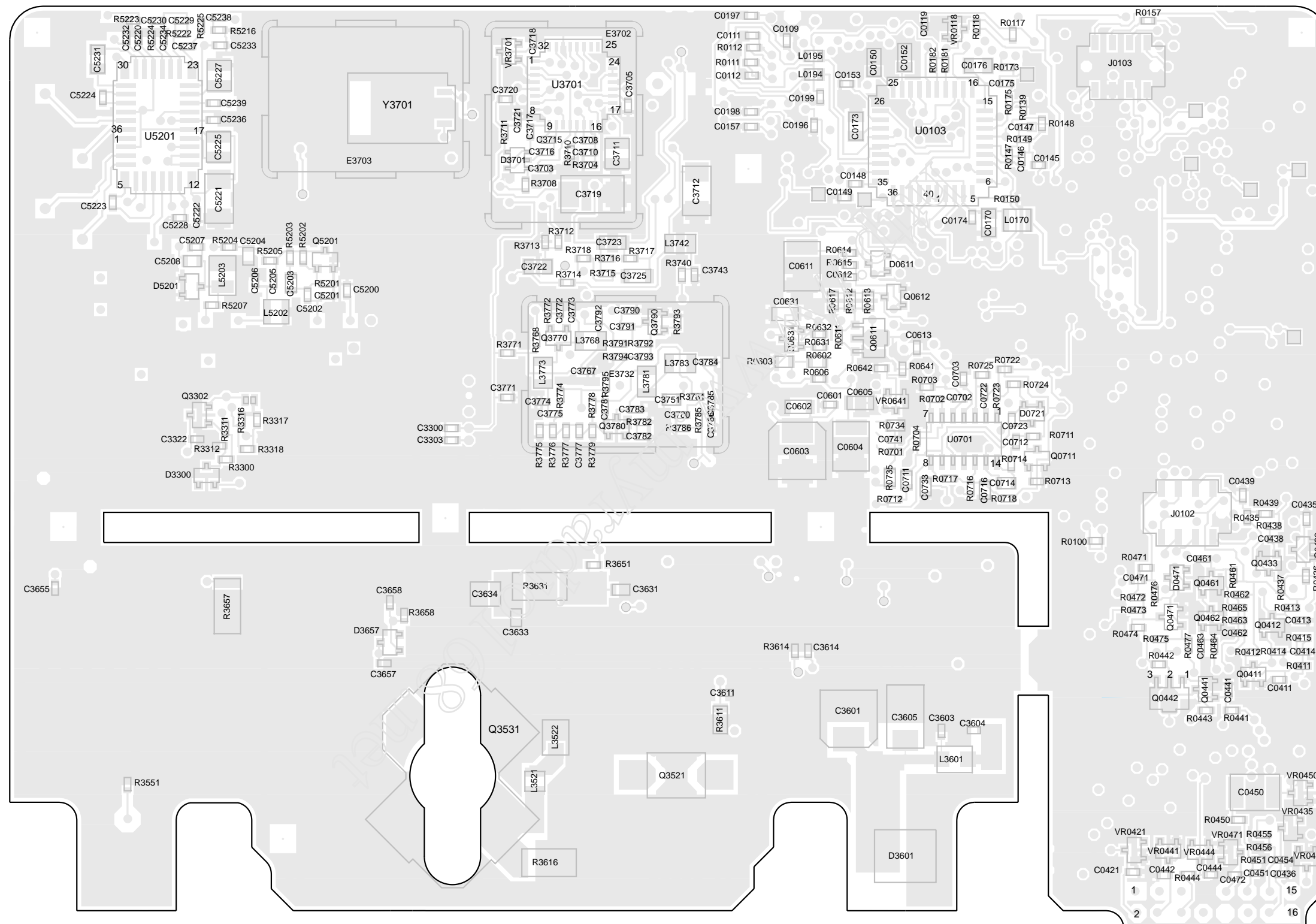
VHF Main Board Solder Side PCB No. 8405669Z01
