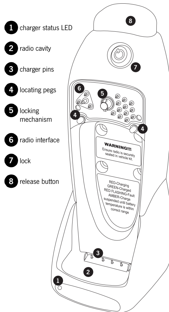
Figure F-6: Vehicle kit assembly
