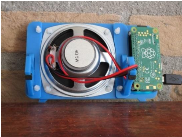
Figure 46 Pimoroni Pirate Radio - Rear view
