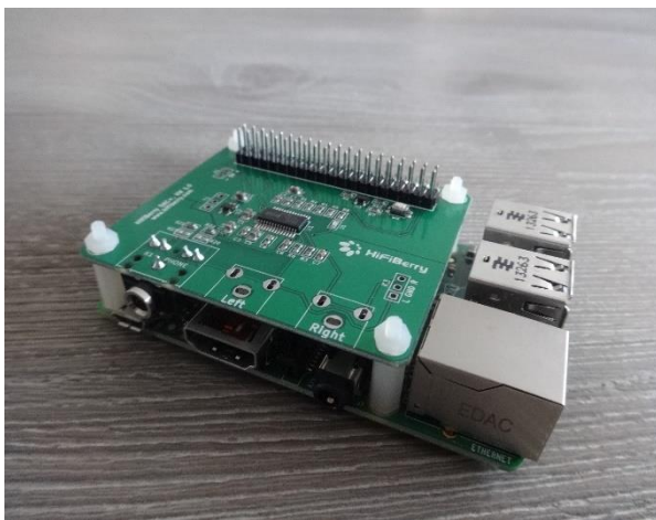
Figure 95 HiFiBerry mounted on the Raspberry Pi
