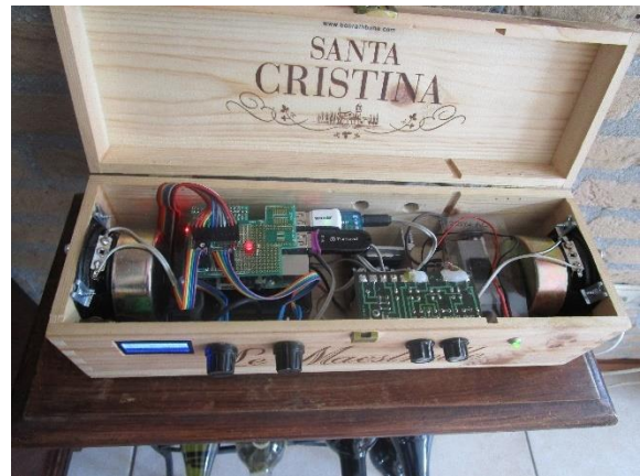
Figure 16 Wine box internet radio internal view
