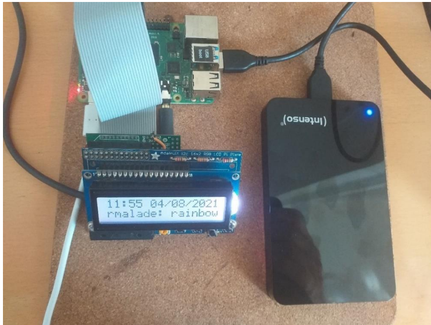
Figure 224 Raspberry Pi booting from an Intenso USB 3.0 2.5-inch disk drive
