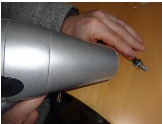
Figure 109 Shrink shrink-wrap with a hair dryer
