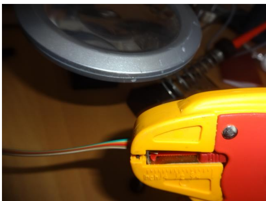
Figure 106 Using wire strippers
