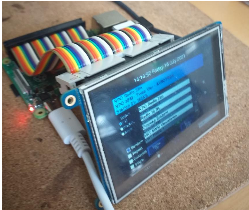
Figure 51 TFT connected by a 40-pin male/female ribbon cable
