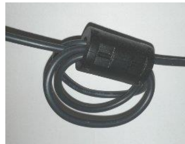
Figure 118 Loop +5V supply around the core
